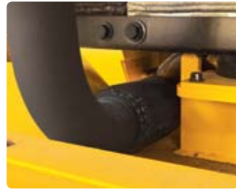
Expansion Bellows The expansion bellows absorbs vibration and reduces noise generated from the exhaust system and also extends the life cycle of exhaust system.
