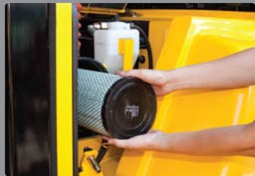
Easy Change Air Cleaner The air filter is readily accessible for cleaning or replacement.
