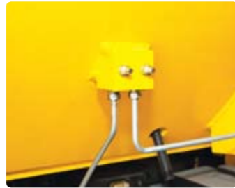
Grease Fittings Grease fittings are installed for fast access to steering axle center pin when doing your service checks.
